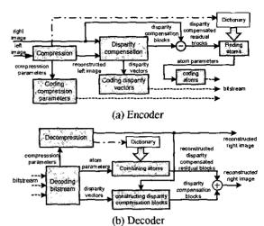
Fig.2 A stereo image coding system using Two-stage Orthogonal Matching Pursuit (TSOMP)
