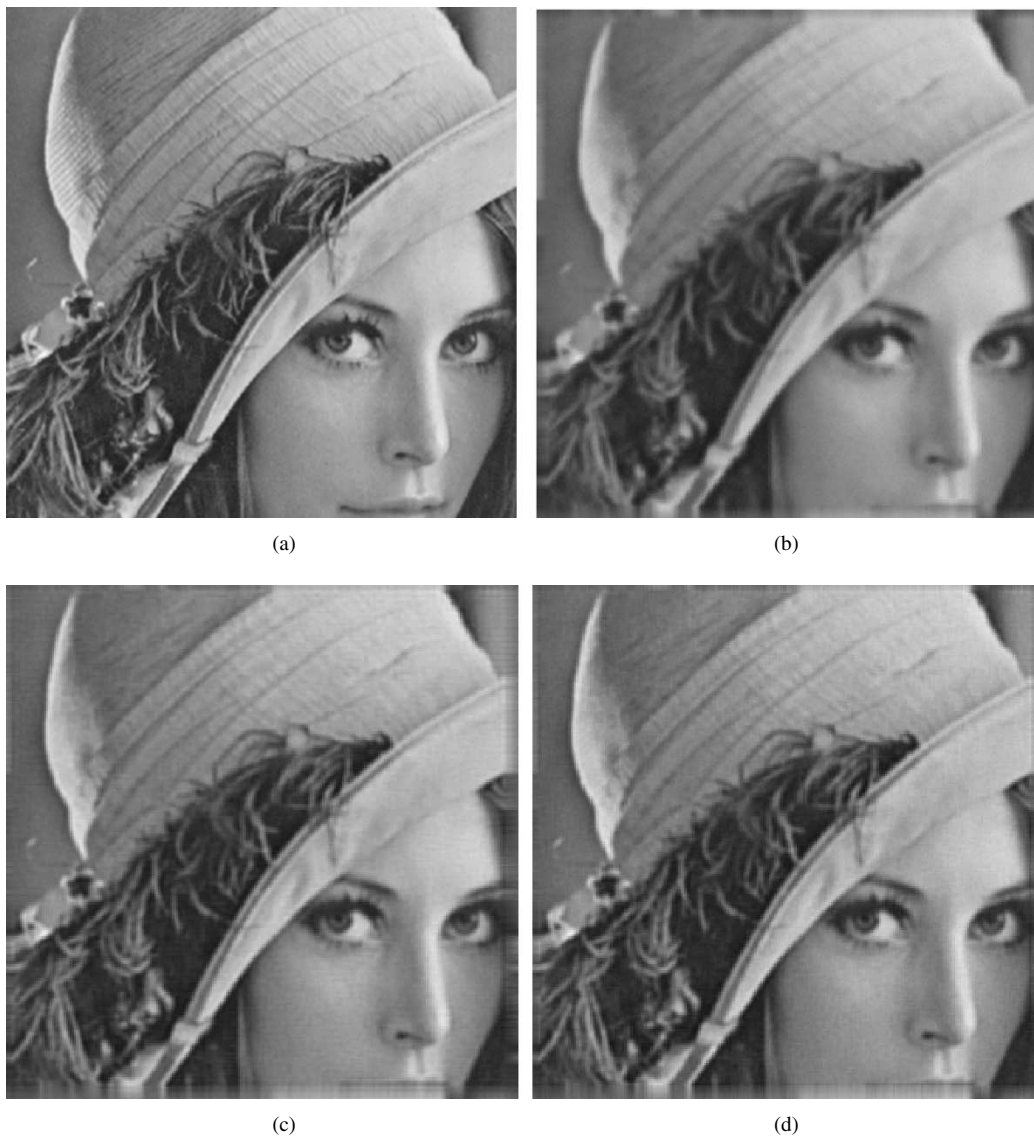
Fig. 4. (a) Original Lena ( 256 \times 256 ). (b) Blurred and noisy Lena ( \text{BSNR} = 30 dB). (c) Restored Lena using 2-D GCV ( \text{SER} = 27.13 dB). (d) Restored Lena using the proposed DPRT approach ( \text{SER} = 27.86 dB).
