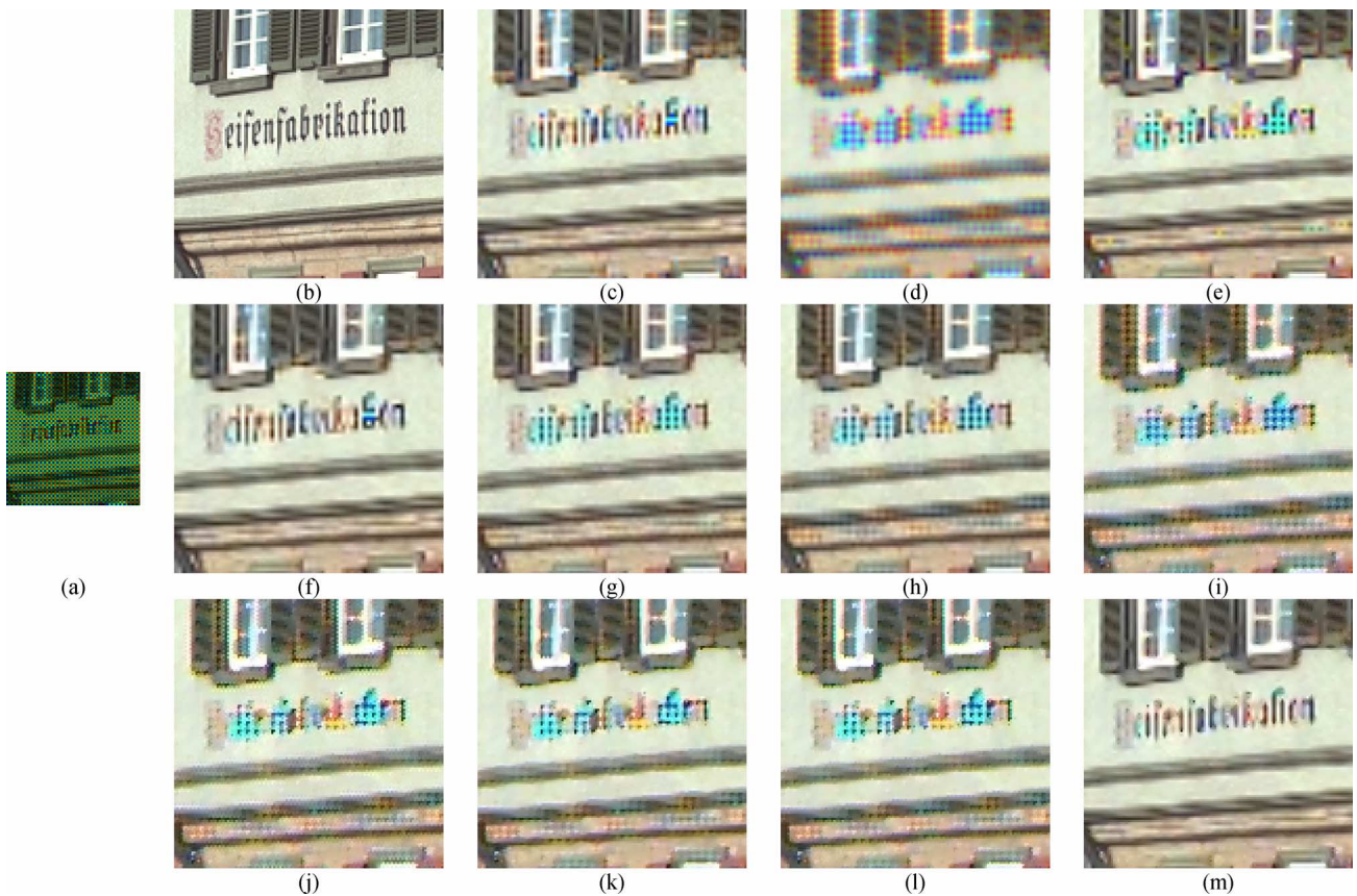
Fig. 10. Part of the processing results of image 8: (a) the input CFA image, (b) the full-color original, (c) PCSD+BI, (d) BICD+BI, (e) ACPI+BI, (f) AHDA+BI, (g) AP+BI, (h) NCED+BI, (i) DCZPS, (j) CIZBP+AP, (k) CIZBP+AHDA, (l) CIZBP+NCED, and (m) the proposed algorithm.
