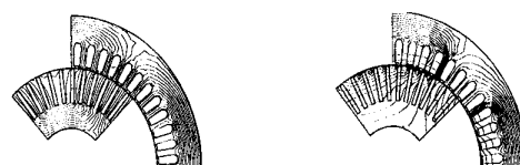
(a) With both a.c. and d.c. exciting Difference between lines: 2.21 \times 10^{-3} Wb/M (b) With only d.c. exciting Difference between lines: 0.22 \times 10^{-3} Wb/M Fig. 7 Flux distribution for phantom loading with the d.c. current in the ratio of 1:1:0
