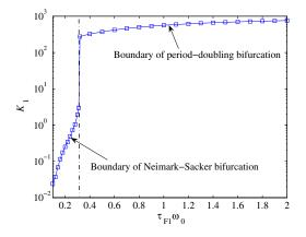
Fig. 4. Boundaries of slow-scale and fast-scale bifurcations for  $K_i = 1$ . The dash line shows the boundary between the two types of bifurcation.
