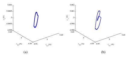
Fig. 3. 3-dimensional trajectories. (a) Stable period-one trajectory for  $K_1 = K_2 = 560.5$ ,  $\tau_{F1} = \tau_{F2} = 1/\omega_0$ ,  $K_i = 1$ ; (b) period-2 trajectory after the fast-scale bifurcation for  $K_1 = K_2 = 561$ ,  $\tau_{F1} = \tau_{F2} = 1/\omega_0$ ,  $K_i = 1$ .
