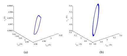
Fig. 2. 3-dimensional trajectories. (a) Stable period-1 trajectory for  $K_1 = K_2 = 1.9$ ,  $\tau_{F1} = \tau_{F2} = 0.3/\omega_0$ ,  $K_i = 1$ ; (b) quasi-periodic trajectory after the slow-scale bifurcation for  $K_1 = K_2 = 2$ ,  $\tau_{F1} = \tau_{F2} = 0.3/\omega_0$ ,  $K_i = 1$ .
