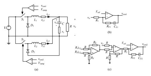
Fig. 1. Parallel connected buck converters under master-slave current sharing and PI control. (a) Converter stage; (b) controller for the master; (c) controller for the slave.
