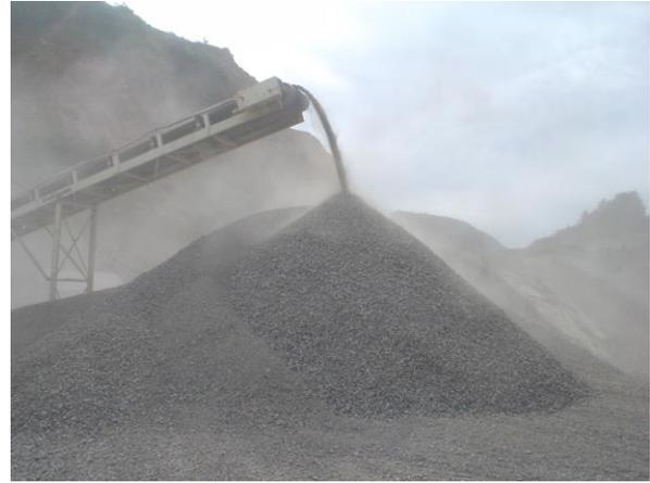
**Figura 13.** Chorro de material principal (base o sub-base).
