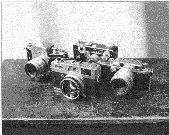
Fig. 5. High Resolution Scan. Image captured on 200 ISO film and scanned with a Nikon LS-100 negative scanner, measuring 2403 x 1918 pixels, producing a 4.6 million pixel image. A Nikon NC2000e digital camera can only capture 1.6 million pixels (1268 x 1012 pixels).
