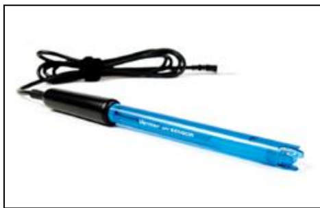
Figura 3.17. Sensor de pH [13]
