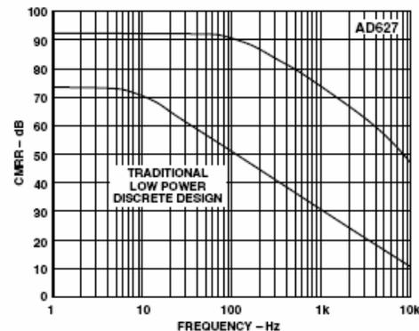
Figure 1. CMRR vs. Frequency,  $\pm$ 5  $V_S$ , Gain = +5
