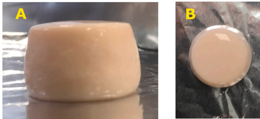
Fig. 3. Side (a) and top (b) view of the gel prepared from the milk protein dispersion using the conditions pH 6.0, [Ca^{2+}] = 1.5 mM, and 40 °C after decreasing the temperature to 15 °C using the cycled-temperature ramp method. The gel was elaborated in the rheometer's bob and cut with a 20 mL syringe with the tip removed.
