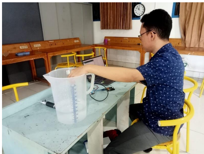
Figure 5. Water Salinity Measurement with TDS Sensor
