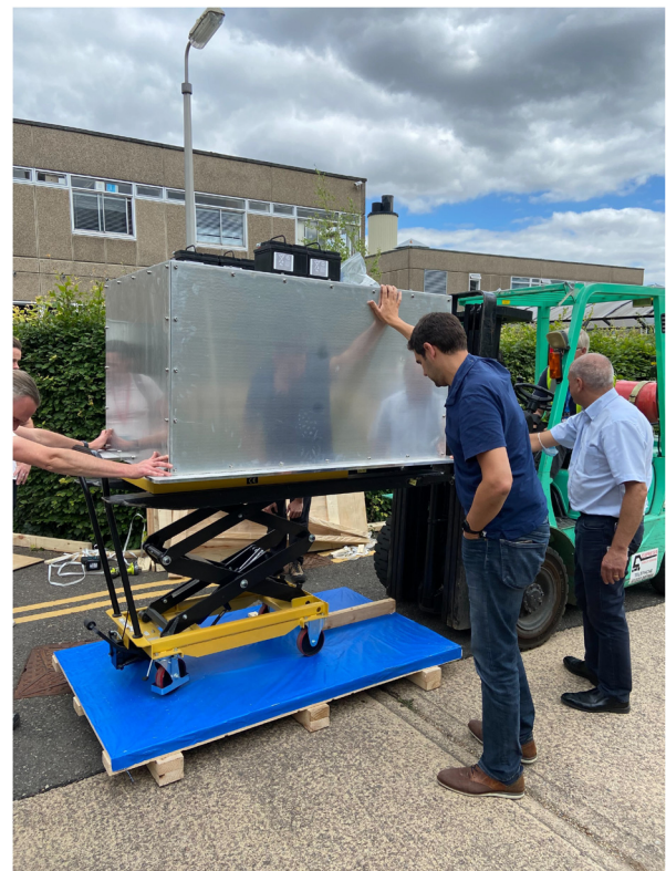
FIG. 7. The University of Cambridge sidearm being unloaded with shearplates in place—showing the transport and assembly trolley and the base of the wooden shipping case.
