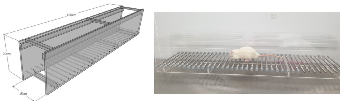
Figure 1. Ladder rung walking apparatus for testing the motor deficit induced by 1-methyl-4-phenyl-1,2,3,6-tetrahydropyridine.
