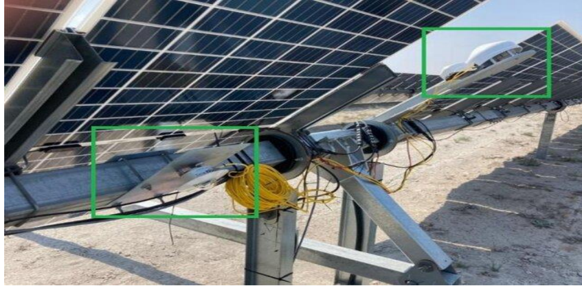
Figure 8. Experimental setup employed for the measurement of spectral albedo; two pyranometers are employed on the panel to measure the back and front solar irradiance.
