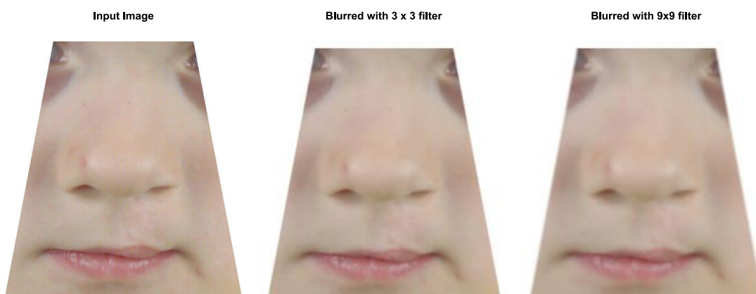
Figure 4. 3: Denoising using the Gaussian approach with different filter sizes of 3 (middle) and 9 (right).
