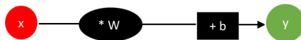
Figure 6. 4: Model Weight intuition. Every feature has a weight (level of importance) attached to it, numerically and a bias to regulate (normalise or 'balance up') the outcome.
