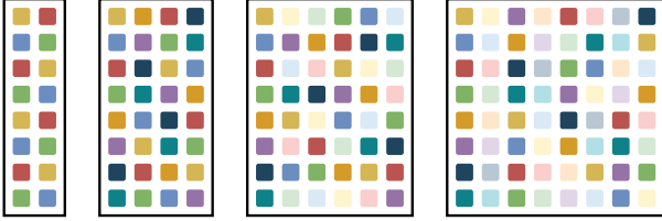
Fig. 2. Optimized grouping for RISs with 2 \times 8 , 4 \times 8 , 6 \times 8 , and 8 \times 8 elements and group size 4.
