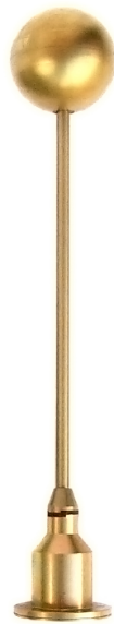
Figure 1.11: One of two spherical Langmuir probes on board ESA's space vehicle Rosetta, due for a comet. Image Credit: ESA/Rosetta Mission/Swedish Institute of Space Physics in Uppsala
