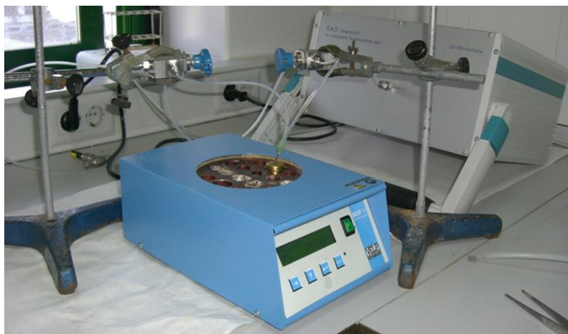
Fig. 2. Photo of the headspace set-up coupled to the UV-IMS.
