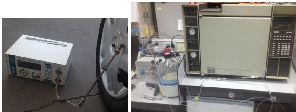
Fig. 6. Photo of the adsorption step with the extraction pump and TENAX column and desorption step of TENAX column performed in a GC oven coupled to UV-IMS.
