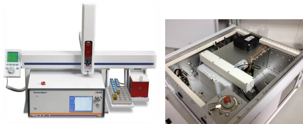
Fig. 9. Photo of the FlavourSpec® used from GAS and internal detail of the instrument.
