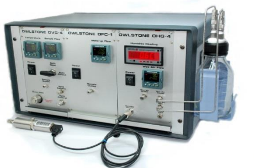
Fig. 5. Photo of the calibration gas generator from Owlstone ® used.
