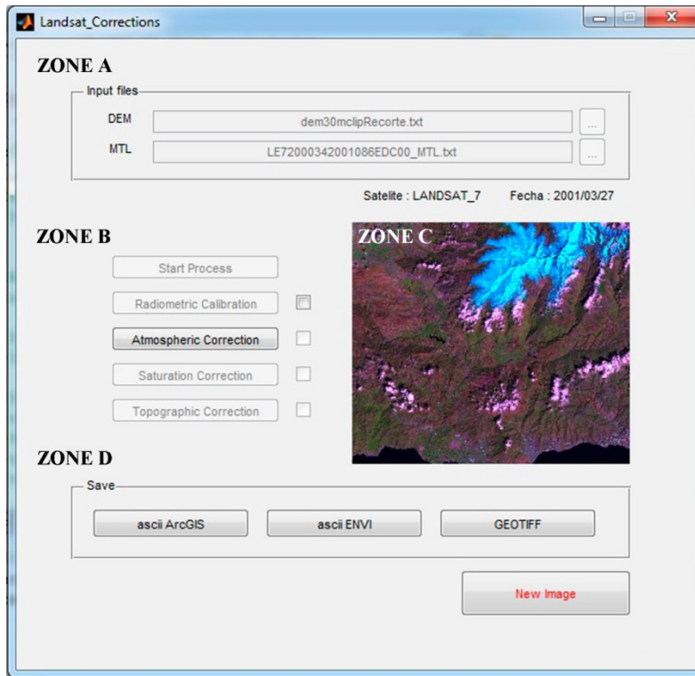
Figure B.2 GUI tool for preprocessing Landsat images. Four zones can be distinguished: ZONE A, where the two inputs are loaded; ZONE B, area where the different preprocessing steps can be selected; ZONE C, where the selected area of the Landsat scene and some data are visualized; and ZONE D, area where the different output format can be selected.
