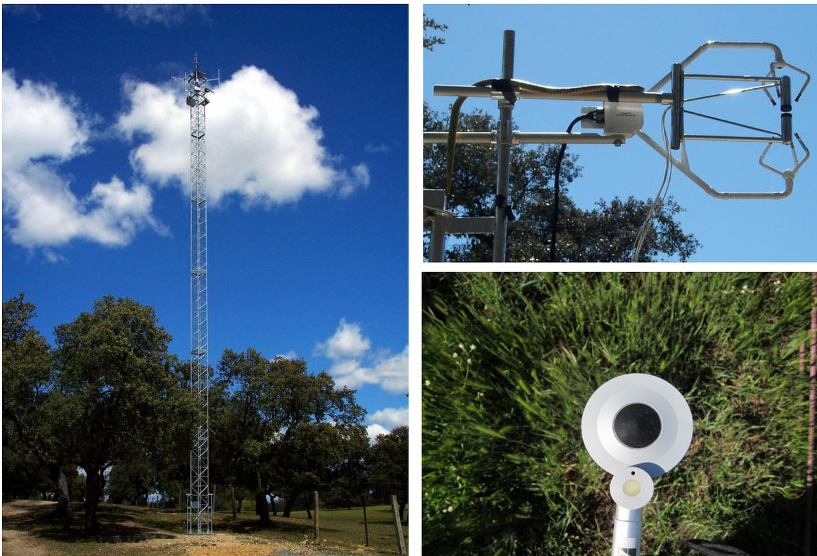
Figure 2.4: ECT installed in Santa Clotilde study area. CSAT 3D, KH20 and net radiometer over the grass.
