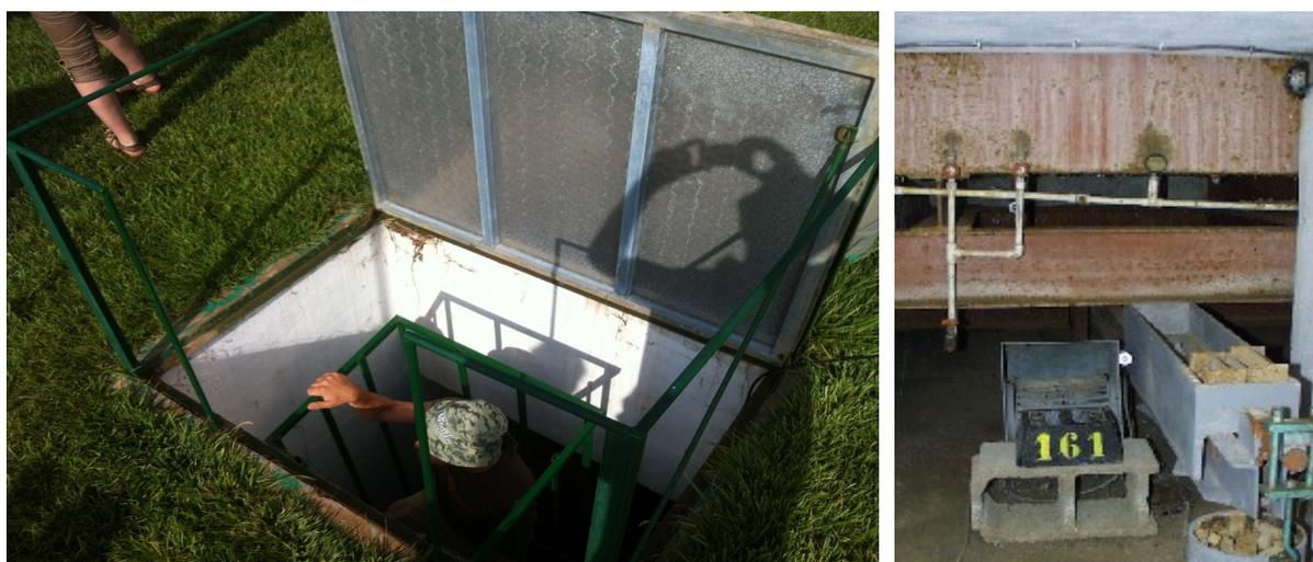
Figure 1.6: Lysimeter system located in Las Tiasas experimental farm, outside and inside equipment (Source: Instituto Técnico Agronómico Provincial, ITAP, Barrax, Albacete, Spain. During REFLEX training course).
