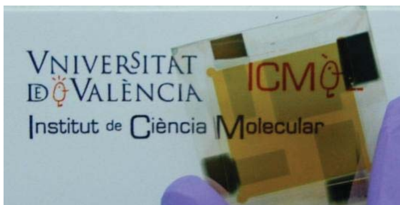
Fig. 5.13 Photograph of the semitransparent solar cell having a 100 nm perovskite layer resulting in an AVT \sim 30% and a PCE of 6.4%.
