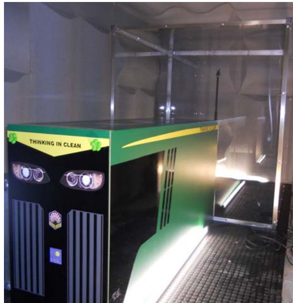
Figure 5.2. Photo of the experimental setup: vibro-acoustic cabin mock-up inside the semi-anechoic chamber
