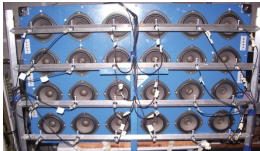
Figure 4.5. Loudspeaker cabinet and microphone array
