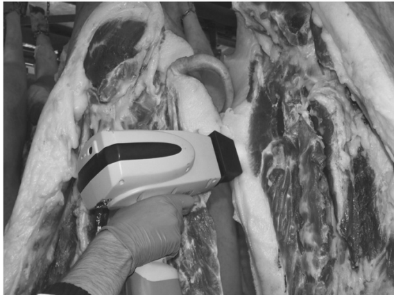
Fig. 1. In-situ NIRS carcass analysis performed with a handheld MEMS instrument.
