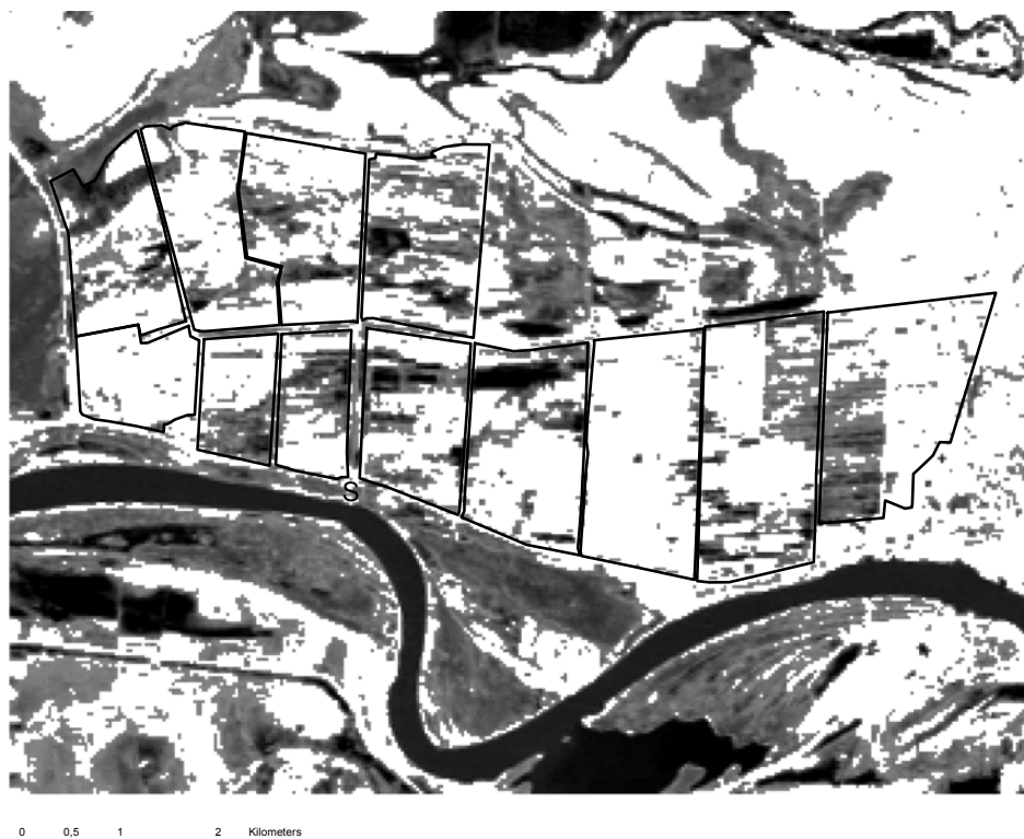
Figure 5.7. Map of drainage problems based on infrared reflectance measured from Landsat satellite over M'Pourie irrigation scheme.
