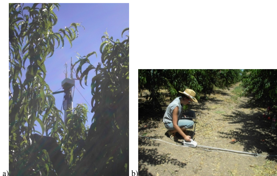
Figure 1.2. Sensor measuring PAR above the canopy (a), and a portable ceptometer device making spot measurements below the canopy (b).
