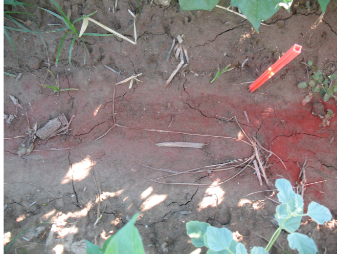
Figure 3.12. Tagged soil redistribution after the irrigation test in an intermediate furrow segment tagged with hematite.
