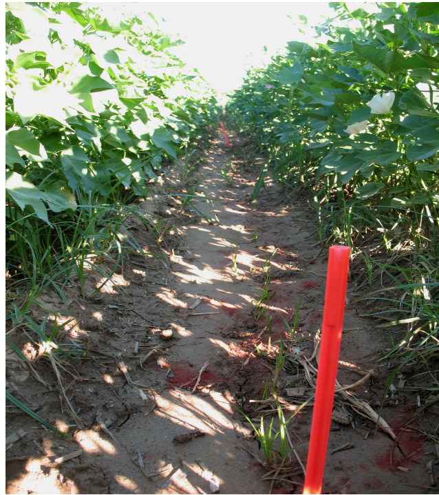
Figure 3.14. Intermediate tagged segment with hematite, after the rain simulation test, where tracer losses and deposition of untagged sediments are visible.
