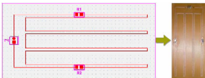
Fig. 7. Passive voltage divisor in a printed circuit board designed (badly) in CADSTAR
