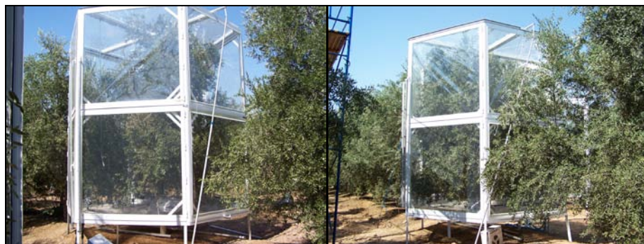
Fig 5. Before measuring, the windows and top are closed and fans turned on. The \text{CO}_2 and water vapour concentrations, measured by the IRGA, change steadily after a short lag time. The rate of change of both gases with time is the apparent flux of assimilation or respiration and transpiration, respectively, of the tree. After the measurement is completed, the chamber goes back to the open position as Fig. 4, with the fans off until the following measurement.
