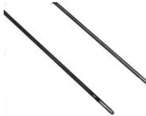
Fig. 2. Cathodes after arcing with a mixture of argon and hydrogen (cathode at top of the photograph) or with pure argon (cathode at bottom of the photograph) as the plasma-forming gas. A ring-shaped layer of oxide at 12 mm from cathode's tip can be seen in the latter cathode. The EDX analysis indicated the following atomic composition at a point on this layer: 34.34% O, 0.24% Th, 20.18% W, and 45.24% C. Off the layer the composition is: 25.45% O, 0.32% Th, 24.15% W, and 50.08% C at a point closer to the tip, and 22.88% O, 0.51% Th, 17.64% W, and 58.97% C at a point further away from the tip. The EDX analysis of the lateral surface of the cathode used with a mixture of argon and hydrogen gave the following atomic composition: 2.89% O, 1.74% Th, 86.88% W, and 8.49% C.
