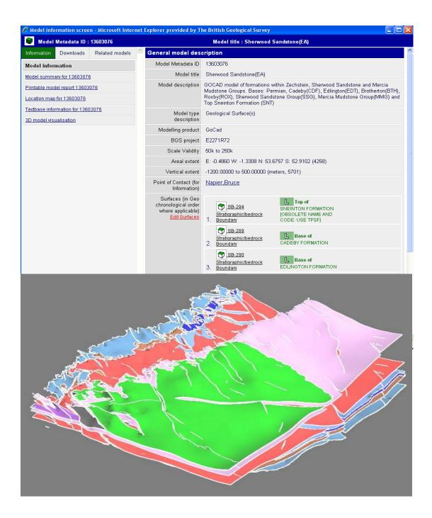
Figure 7. 3-dimensional geological model of part of central England, constructed using GoCAD software to assist with groundwater management applications. Approximate model dimensions 75km. x 30 km. x 0.4 km. Metadata screen illustrates discovery metadata for whole model. More detailed DGSM metadata for each stratigraphic surface and groups of faults can be selected and interrogated individually.
