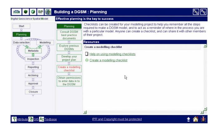
Figure 8. Screenshot example of web-based interface to BGS Digital Geoscience Spatial Model workflow application, illustrating main workflow tasks and sub-tasks. Clicking on each link in workflow takes user to best practice documents that recommend methodologies to be used for each task. A checklist is then automatically populated and stored along with metadata for each model, recording practices used.
