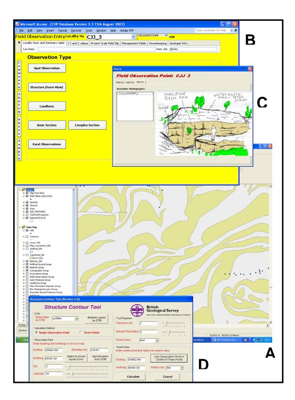
Figure 5. Montage of screenshots showing examples of data entry, notes and sketches 'pages' in BGS MIDAS digital field data recording application. A. 'Digital field map' interface with digital geological map backdrop; B. Launch screen for 'digital field notebook' application; C. Data review screen showing sketch captured at a field locality; D. Application for predicting outcrop position of a dipping surface based on a structural dip measurement or three known points.
