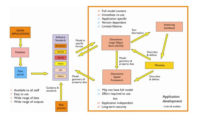
Figure 6. Data, information and knowledge flow within BGS Digital Geoscience Spatial Model system (after Smith, 2005). EarthVision, GSI3D, GoCAD and Vulcan are various third party 3D modeling software packages used by BGS during development and testing of DGSM system.
