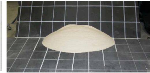
Figure 6. Physical Modeling of Runout/Pileup of Rock Avalanche. (from Manzella and Labiouse. 2007, 2008)
