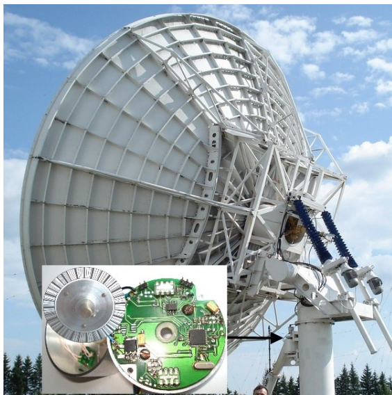
Figure 5. Experimental sample of optical-electronic angle sensor and AS "Vityaz-7m" with mounted sensors
