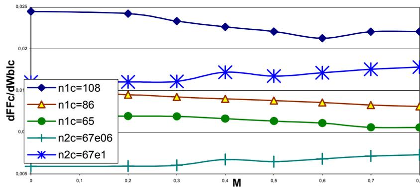
Figure 3. Relation between the derivative  $dFFc/dWb1c$  and the Mach number, at different engine fan rotational speeds in percents and different points of air bleed
