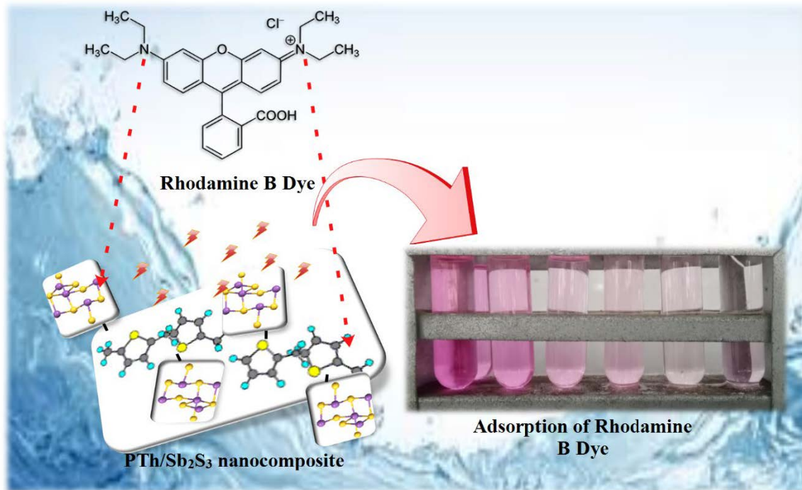
260 Fig.6. Adsorption mechanism of RhB dye at the surface of PTh/Sb 2 S 3 nanocomposite
