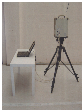
Figure 4: Image of the 3D laser scanner on a tripod connected to a laptop
