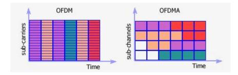
Figure C.2: OFDM/TDMA and OFDMA
