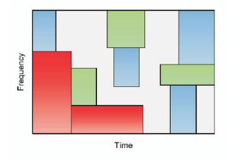
Figure 2.2: Allocation of resources to operators as experienced in position X in figure 1.1. The pink area is vacant for any operator in this position [2]
