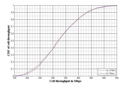
Figure 5.9: CDF of cell throughput: GTBA vs Tmax
