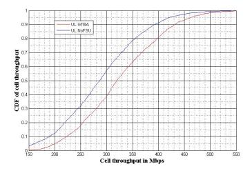
Figure 5.16: CDF of cell throughput: GTBA vs NoFSU
