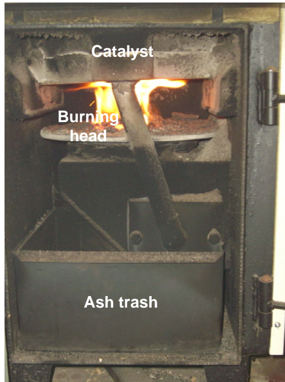
Figure F.4: The burning chamber with the burning head and the catalyst. The pipe going up to the catalyst is the secondary air. The ash trash in the bottom collects the ash from the solid fuel.
