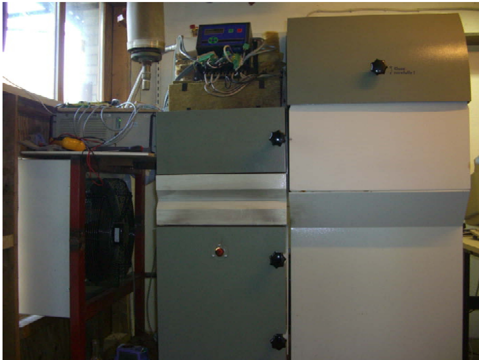
Figure F.1: The whole test set up. The load can be seen to the left and the target PC is just above the load. The lowest chamber in the middle is the burning chamber and the one above is the gas chamber. Just above the gas chamber can the original controller from Techno-Matic A/S be seen. Behind the white plate to the right are the two actuators located and above them is the solid fuel chamber.
