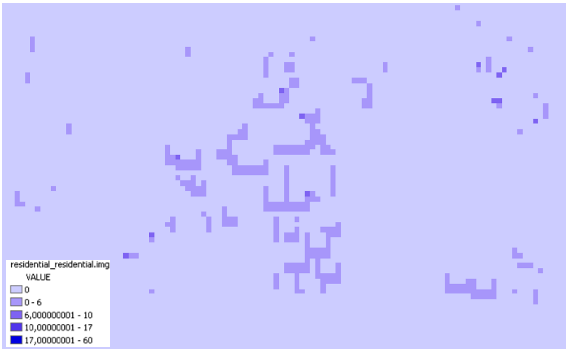
Figure 18b. An example of the ResidentialResidential raster, which includes only the previous FocalSum values of new residential cells . A neighbourhood of 61 cells have been used.
