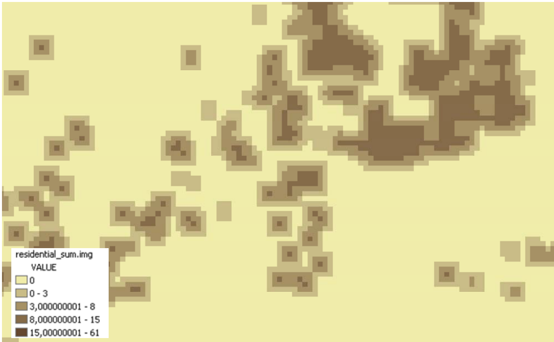
Figure 18a. An example of the FocalSum values of ResidentialSum raster. A neighbourhood of 61 cells have been used.
