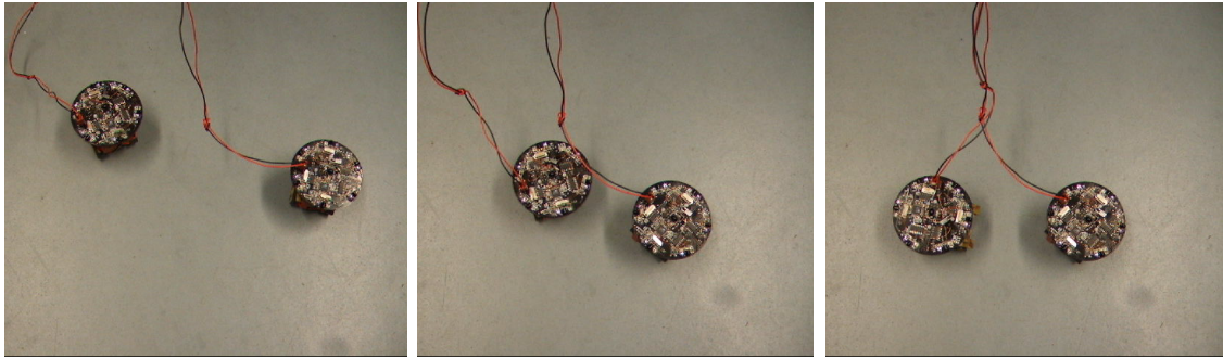
(a) Two robots are moving freely . (b) R0 meets R1 and asks R1 to stop. (c) R0 is adjusting the direction 00to12.
