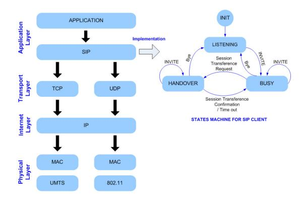
Figure 4.15: States machine and protocol stack
