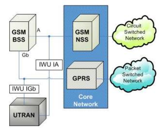
Figure 3.1: UMTS general system architecture
