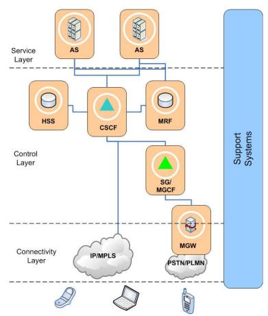
Figure 3.7: Simplified view of the IMS layered architecture in IMS
