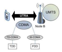
Figure 3.2: UMTS air interface
