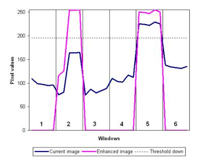
**Figure 3.14:** Brightness enhancement illustration: for each window, pixel values are normalized so that darker areas are not automatically discarded. The multiplication's factor is thresholded ( $\varepsilon$ ) to prevent dark zones without fingers from being enhanced
