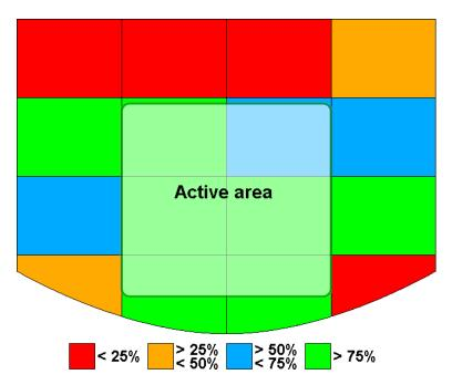
Figure 6.3: Finger detection test's final result: the application's active area matches the surface's areas with high finger recognition rate
