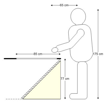
Figure 4.12: Table dimension issue: for a user standing in a natural position, the furthest surface's areas are difficult to reach
