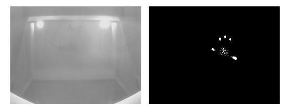
Figure 4.8: Subtraction including binarization example: the current image's pixels (*right image*) that differ from the reference image's ones (*left image*) are set to 255
