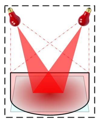
Figure 4.11: Active area illustration: the center of the surface (dark red zone) offers the highest level of infrared light
