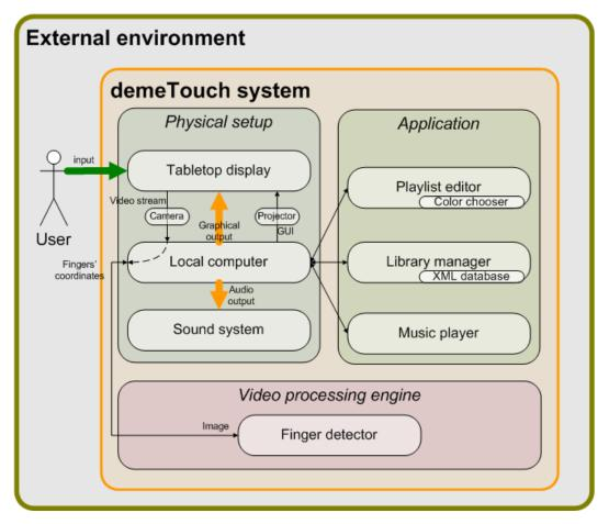
Figure 4.2: The three subsystems involved in demeTouch
