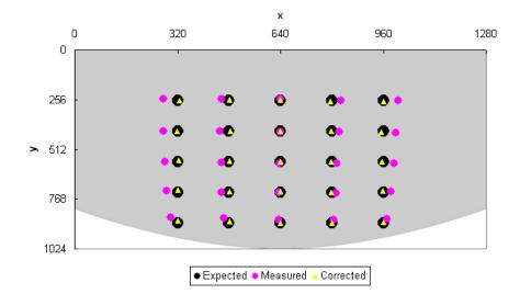
Figure 4.18: Corrected coordinates using general solution in ideal configuration
