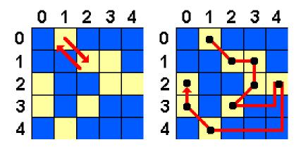
Figure 3.16: Spot creation's process: marking pixels while adding them to the spot prevent from entering in a infinite loop (*left image*) when the connected pixels are considered
