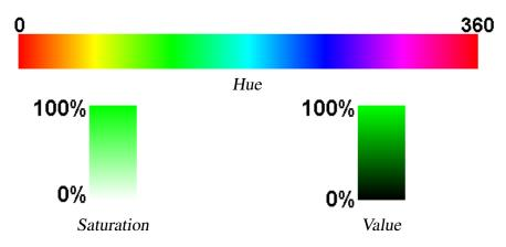
Figure 4.23: The HSV model's three parameters. Saturation and value are shown for hue=120
