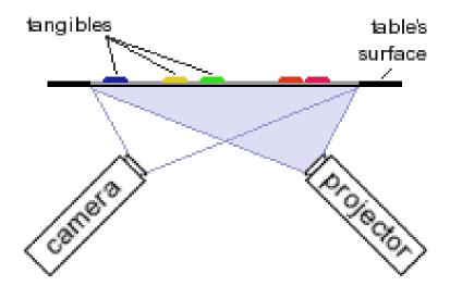
Figure 2.4: The table design (simplified): information exchanged between the table's surface and the computer vision engine are bidirectional
