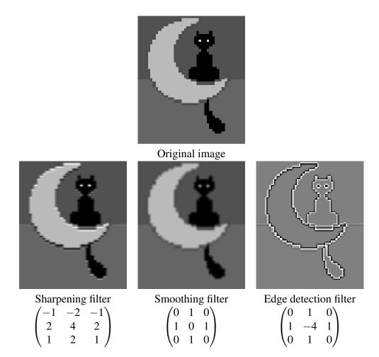
Figure 3.6: Three examples of convolution applied to the same image. For each example, the corresponding kernel is indicated
