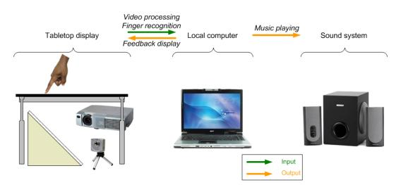
Figure 4.1: The three physical components and their interaction
