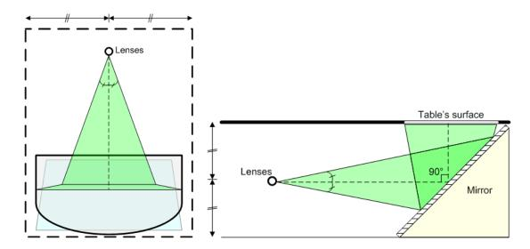
Figure 3.17: Ideal table setup: placing the camera and the projector in the ideal central position horizontally (*left image*) and vertically (*right image*) limits the distortion angle
