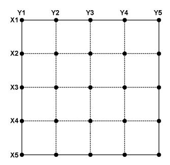
Figure 4.16: Calibration with square mosaic: the coordinates in the camera's system are recorded and confronted to the known values in the projector's coordinates system
