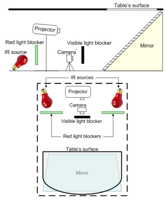
**Figure 4.4:** Final setup of the tabletop display with infrared system, from the side (*top image*) and from above (*bottom image*). (\*) The camera is infrared light sensitive
