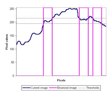
Figure 3.13: Binarization illustration: pixel values are set to 255 only if they are comprised between the two thresholds
