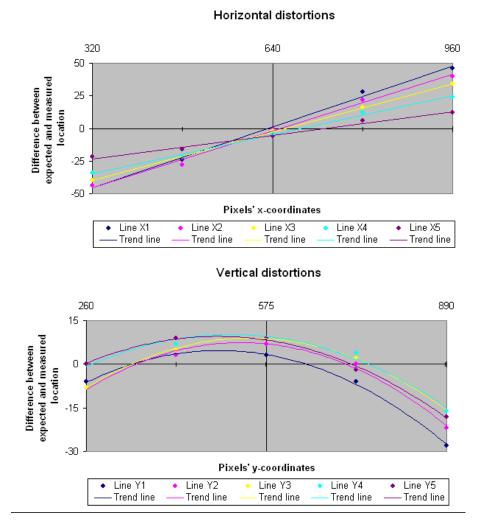
**Figure 4.15:** Distortions representation: the *top image* illustrates the distortion along the x-axis, while the *bottom image* illustrates the distortion along the y-axis
