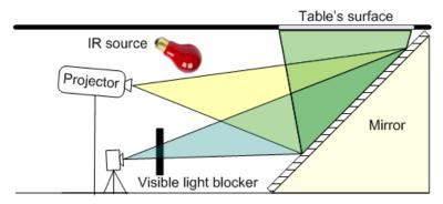
Figure 2.5: The table design (real), including a mirror, infrared sources and visible light blocker
