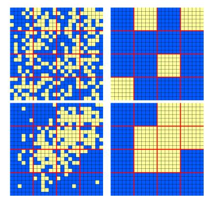
**Figure 3.15:** Holes' removal process: the extremely noisy spot in the *top left* image results in the discontinuous shape (*top right*), while the finger-like spot (*bottom left*) results in the well defined continuous area (*bottom right*)
