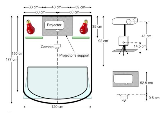
Figure 5.1: The precise measures which make the physical setup easy to repeat
