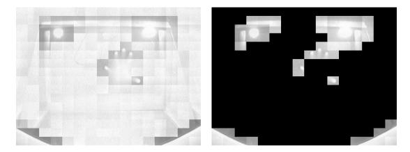
**Figure 4.7:** Brightness enhancement illustration: the current image's brightness is enhanced in every windows first without thresholding the multiplication factor (*left image*). Then the multiplication factor's threshold  $\varepsilon_{Br} = 1.3$  is introduced (*right image*): only windows containing bright spots are kept from the current image
