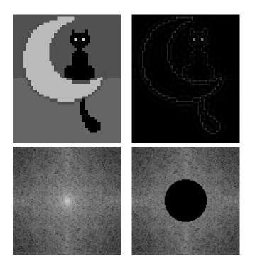
Figure 3.7: An example of edge detection using Fourier transform
