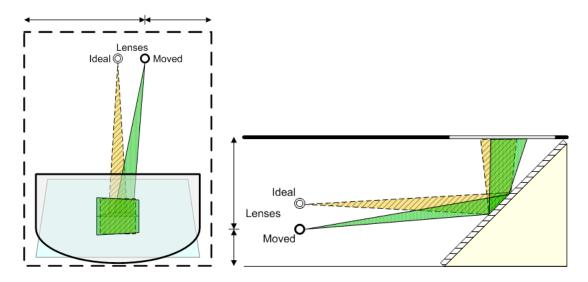
Figure 3.18: Distortion issue: moving the lenses horizontally or vertically from the ideal position introduces an angle that leads to imprecisions in finger recognition
