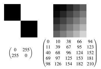
Figure 3.2: Images are represented as an array of pixel values. Here are two examples with their corresponding array representation.
