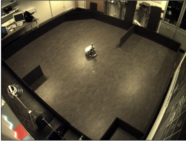
FIGURE 4.1: Still picture captured from the camera surveiling the real-world test environment. Using a wide-angle 4 mm lens ensures full test space coverage.
