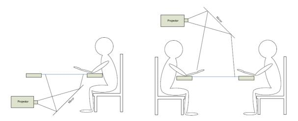
Fig. 2.1.1: Tabletop, side view, bottom and top projection
