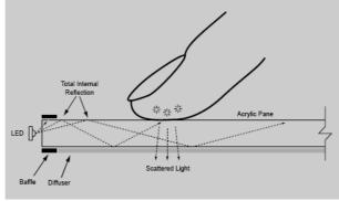
Fig. 1.1.2: FTIR glass side view [3]
