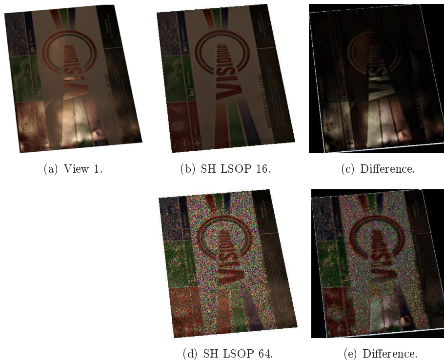
Figure 16.6: A comparison between the real and reconstructed flyer from the first view direction using 16 and 64 parameters in the SH LSOP model.
