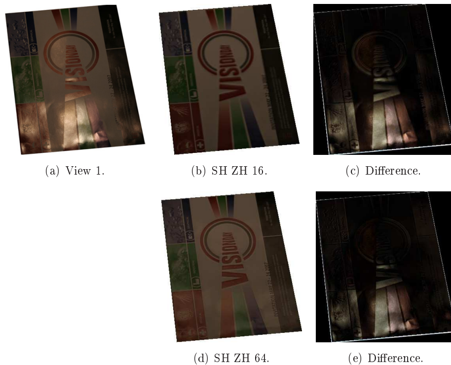
Figure 16.5: A comparison between the real and reconstructed flyer from the first view direction using 16 and 64 parameters in the SH ZH model.
