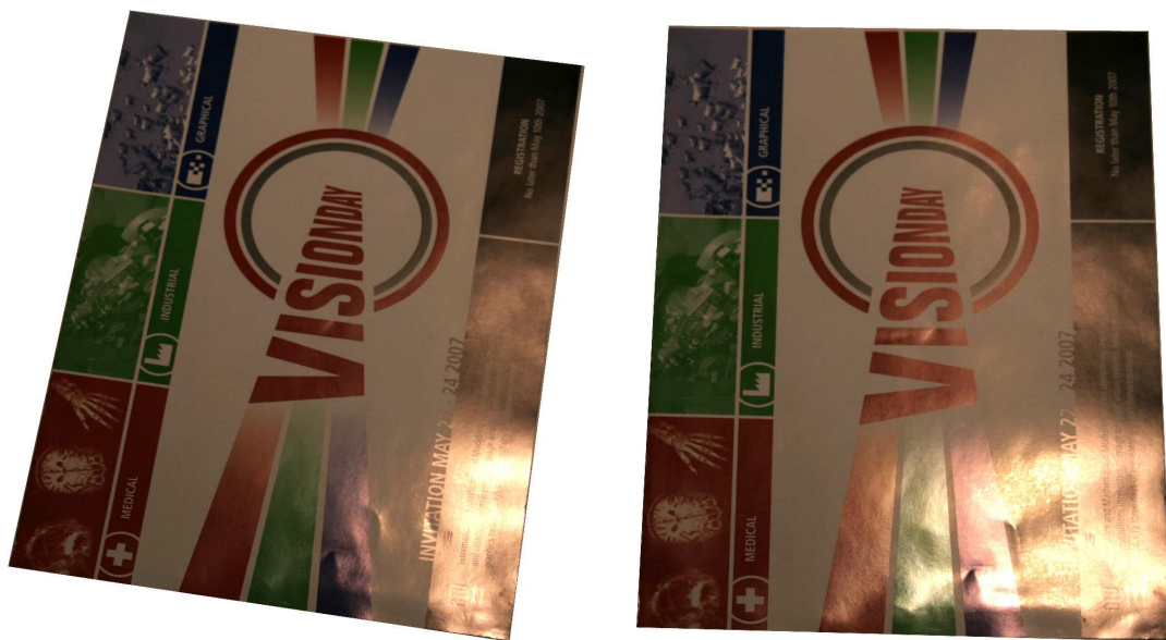
Figure 2.1: Two photographs of the same surface seen from slightly different views with an equal exposure time of 3.2 seconds. The differences are noticeable in subtle material details in the highlights.
