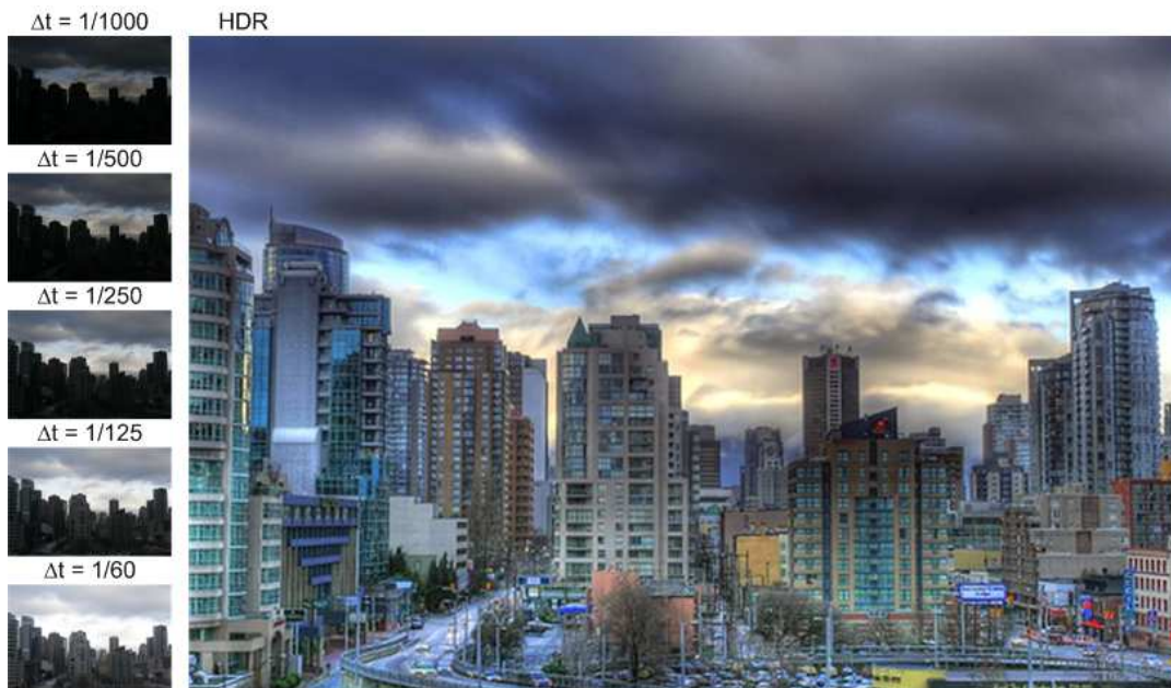
Figure 7.2: An example of a tone mapped HDR image. The five images used to construct the HDR image are shown to the left with their respective exposure time stated above. The HDR image is constructed using Photomatix, and a local tone mapping operator is applied to produce a visually pleasing image with details in both bright and dark areas simultaneously. Images from [Sto].
