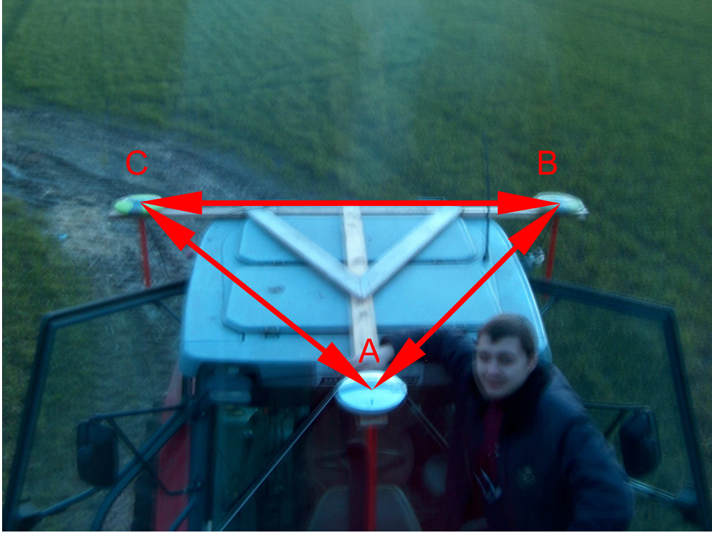
Figure 3.27: Location of GPS antennas on a vehicle
