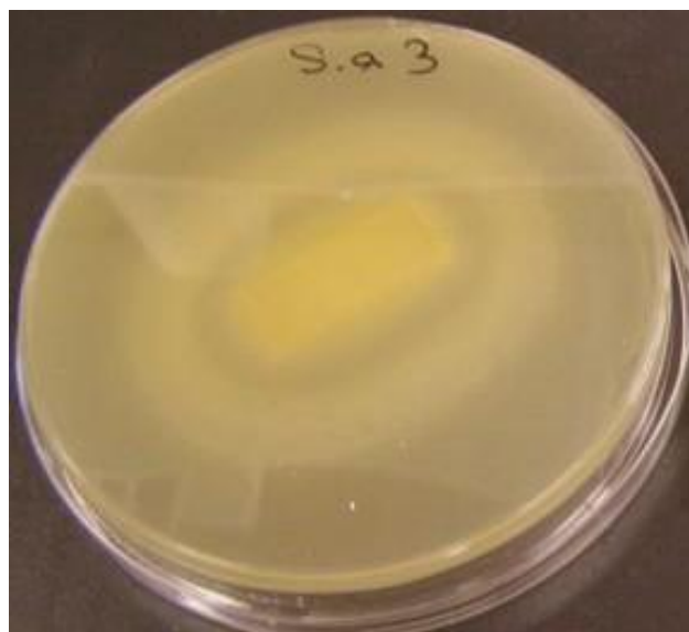
Figure 4.1.4 Microbiological test in selected media (S. Aureus) for wheat gluten/glycerol (WG/G) containing 10 wt.% clove on the inside of the lid.
