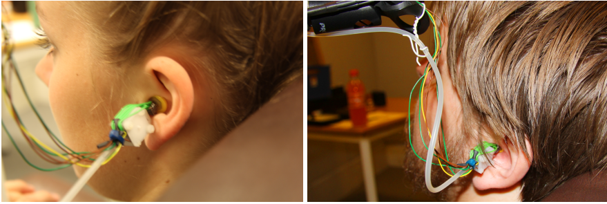
Fig. 2: Custom-built acoustic probe in two subjects for measurement of low-frequency DPOAE. The electroacoustic design is detailed in Paper B and, to some extent, in Paper D. The design is somewhat unfinished but has worked and held its calibration within 1 dB throughout the use in 21 subjects in study D.
