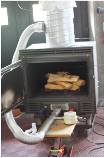
(a) Pre-heated primary air-inlet
