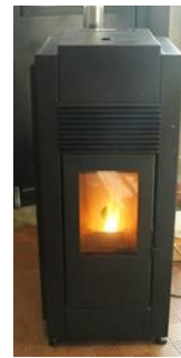
(i) Pellet stove (Digital application) in Portugal.
