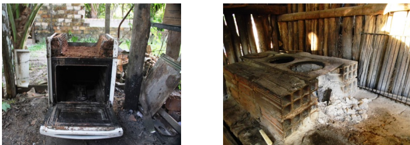
Figure 3-11 Cookstoves in Brazilian houses: reutilization of an LPG stove on the left hand side (a) and a re-framed version of the IDER cookstove on the right hand side (b).
