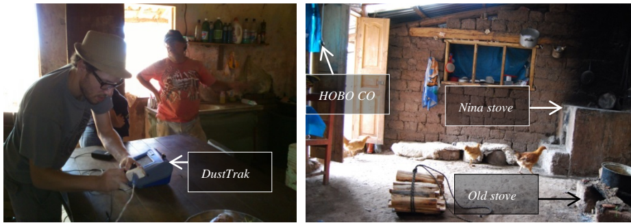
Figure 3-9 Field measurements in a Brazilian house on the left hand side (a) and in a Peruvian setting on the right hand side (b) during the use of ICSs.
