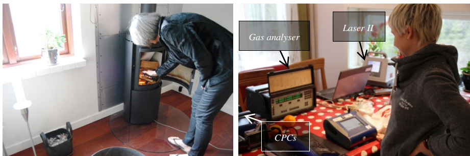
Figure 3-8 Field measurements in a Danish house on the left hand side (a) and in a Norwegian setting on the right hand side (b) during the use of advanced stove applications.
