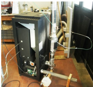
(a) Thermocouples and air-flow meter in the pellet stove
