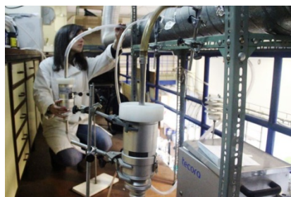
(b) TCR Tecora, sampling probes and filter heads for PM_{2.5}
