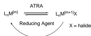
Scheme 5. Catalyst regeneration in metal-mediated ATRA reactions.
