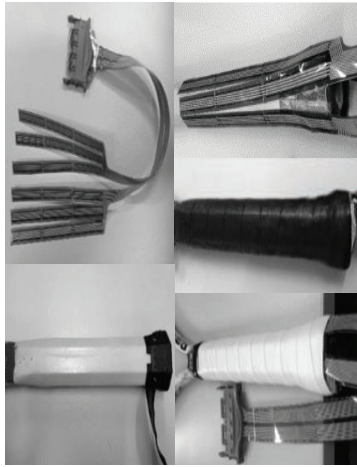
Fig. 1. Modifications of the Tekscan sensor 9811E and the corresponding chronological steps illustrating its application on the grip of the racket handle.
