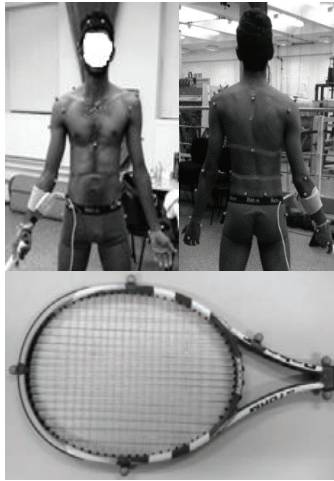
Fig. 2. Tekscan "cuff" attachment, upper body and racket marker protocol.
